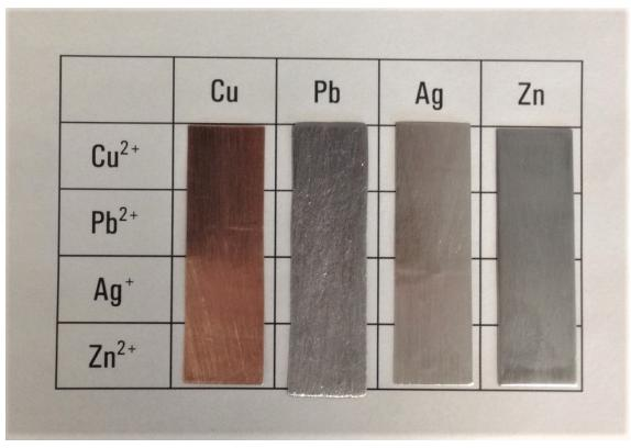
Figure 1: Clean metal strips before applying drops of solutions containing metal ions.
