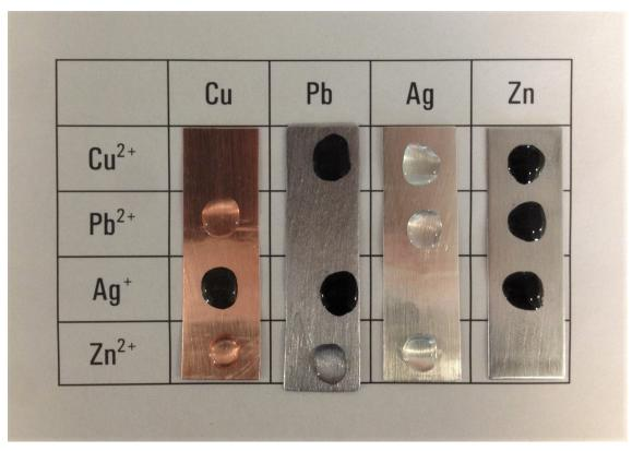
Figure 2: Metal strips after applying drops of solutions containing metal ions.
