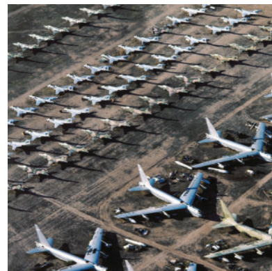
Figure 5 Hundreds of old airplanes are stored at this airplane graveyard in Arizona, U.S., until they can be stripped of any usable parts. The dry desert air prevents the airplanes from rusting.
