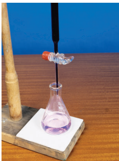
Figure 1 Potassium permanganate is widely used to analyze chemicals that undergo redox reactions, including determining the concentration of iron(II) ions in a sample. When all the iron(II) ions are used up, the solution in the flask turns purple.
