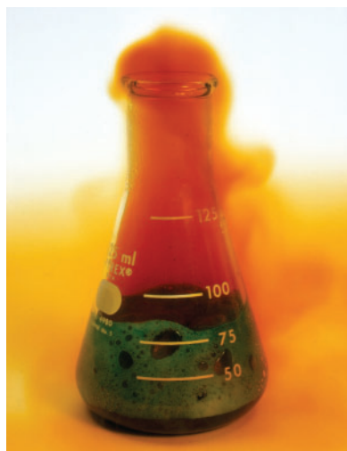
Figure 2 Nitrogen dioxide is a toxic reddish-brown gas produced when concentrated nitric acid oxidizes copper metal.
