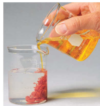
Figure 3 A yellow solution of potassium chromate, \text{K}_2\text{CrO}_4(\text{aq}) , mixes with a colourless solution of silver nitrate, \text{AgNO}_3(\text{aq}) . A reddish-brown precipitate of silver chromate, \text{Ag}_2\text{CrO}_4(\text{s}) , forms as the solutions mix.
