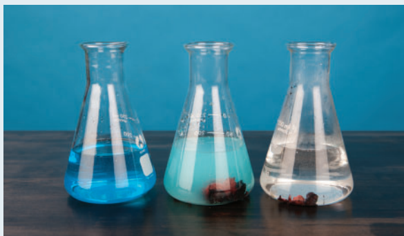
Figure 3 Stages in the reaction progress of elemental zinc in copper(II) chloride solution
