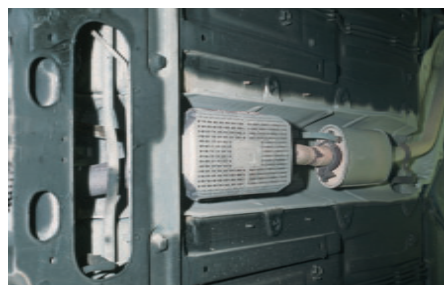
Figure 5 A catalytic converter converts toxic exhaust emissions from an internal combustion engine into non-toxic substances. A thin layer of the metal catalyst is spread over a honeycomb lattice to increase the surface area of the catalyst, further increasing the reaction rate.
