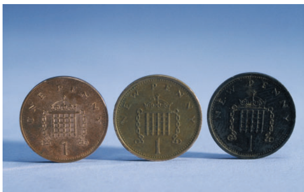
Figure 2 (a) Sodium reacts quickly with oxygen and must be stored covered with mineral oil to avoid exposure to the air. (b) Copper reacts slowly with atmospheric oxygen, forming a layer of brown-black copper oxide. (c) Gold does not oxidize at room temperature—it is resistant to oxidation up to its melting point of 1064 °C.
