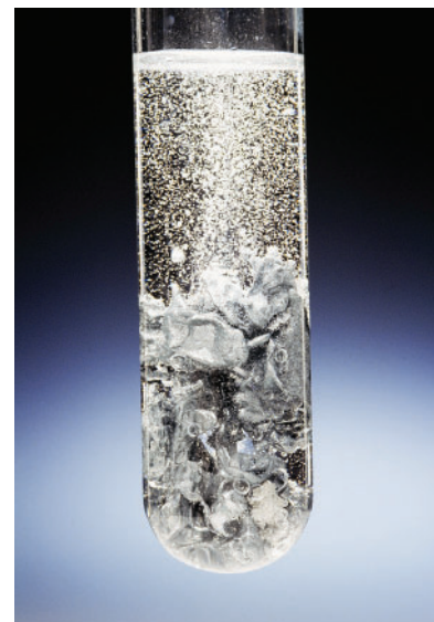
Figure 3 In the reaction between zinc metal and hydrochloric acid, the rate of hydrogen gas formation will increase with the concentration of hydrochloric acid.
