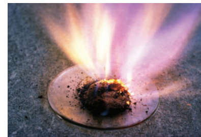
Figure 2 The reaction of potassium permanganate with glycerine. Potassium permanganate reacts so vigorously with most organic compounds, it must be stored separately.
