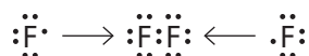
Figure 8 An atom of fluorine has 7 electrons in its valence shell. If it shares one electron with another fluorine atom in a fluorine molecule, each atom will have a total of 8 valence electrons, and become isoelectronic with neon.
